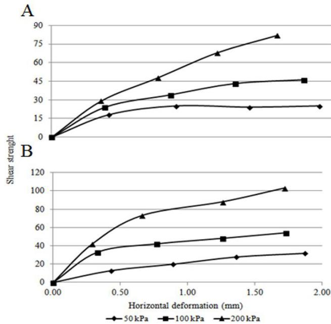
**Figure 3.** Shear strength versus horizontal deformation soil submitted pressure 50, 100 and 200 kPa in the conventional tillage (A) and no-tillage (B).
